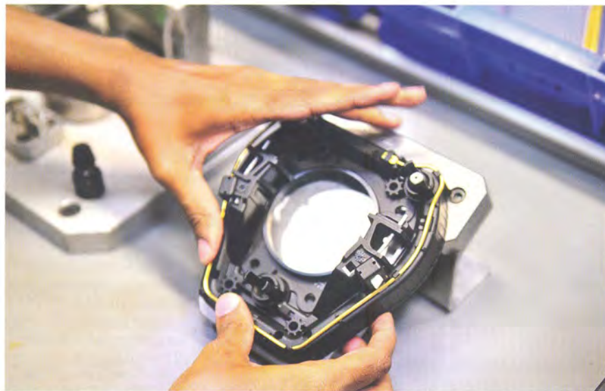
The process of both driver and passenger airbag assembly begins with the housing and logo.
