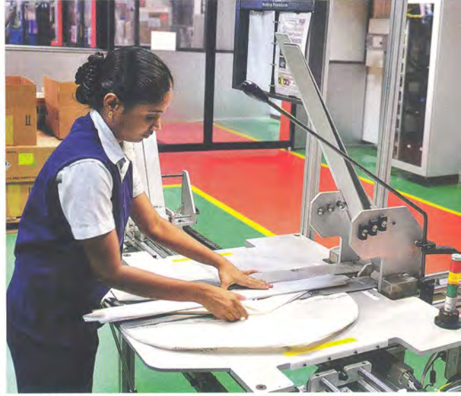
Manual assembly of a passenger airbag on a dedicated line.
