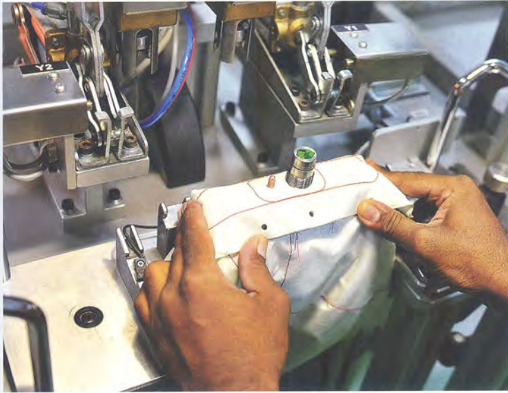
Assembly of the inflator is a key part of the passenger airbag safety process.
