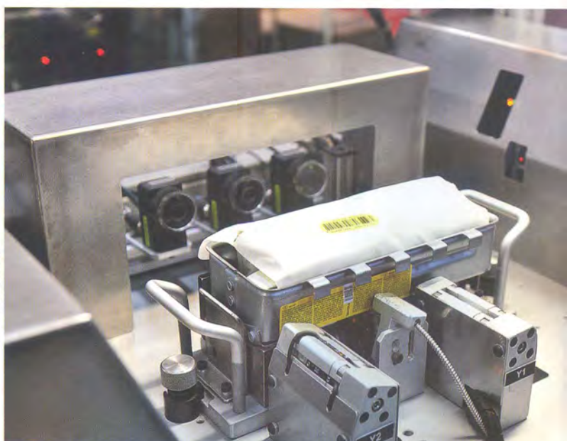
Quality is paramount in the process with one stage involving the use of high-speed cameras to ensure assembly and positioning of all airbag parts are in order.
