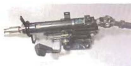
A commercial vehicle steering column assembly. RNSS looking to drive new growth in this segment.
