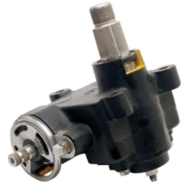
Manual recirculating ball type steering gear
