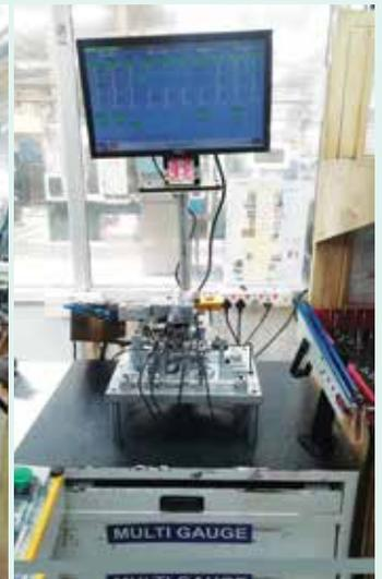
The end-of-line is equipped with digital multi gauging that can inspect and ensure all critical valve parameters simultaneously. Dimensions can be stored and retrieved for analysis.
